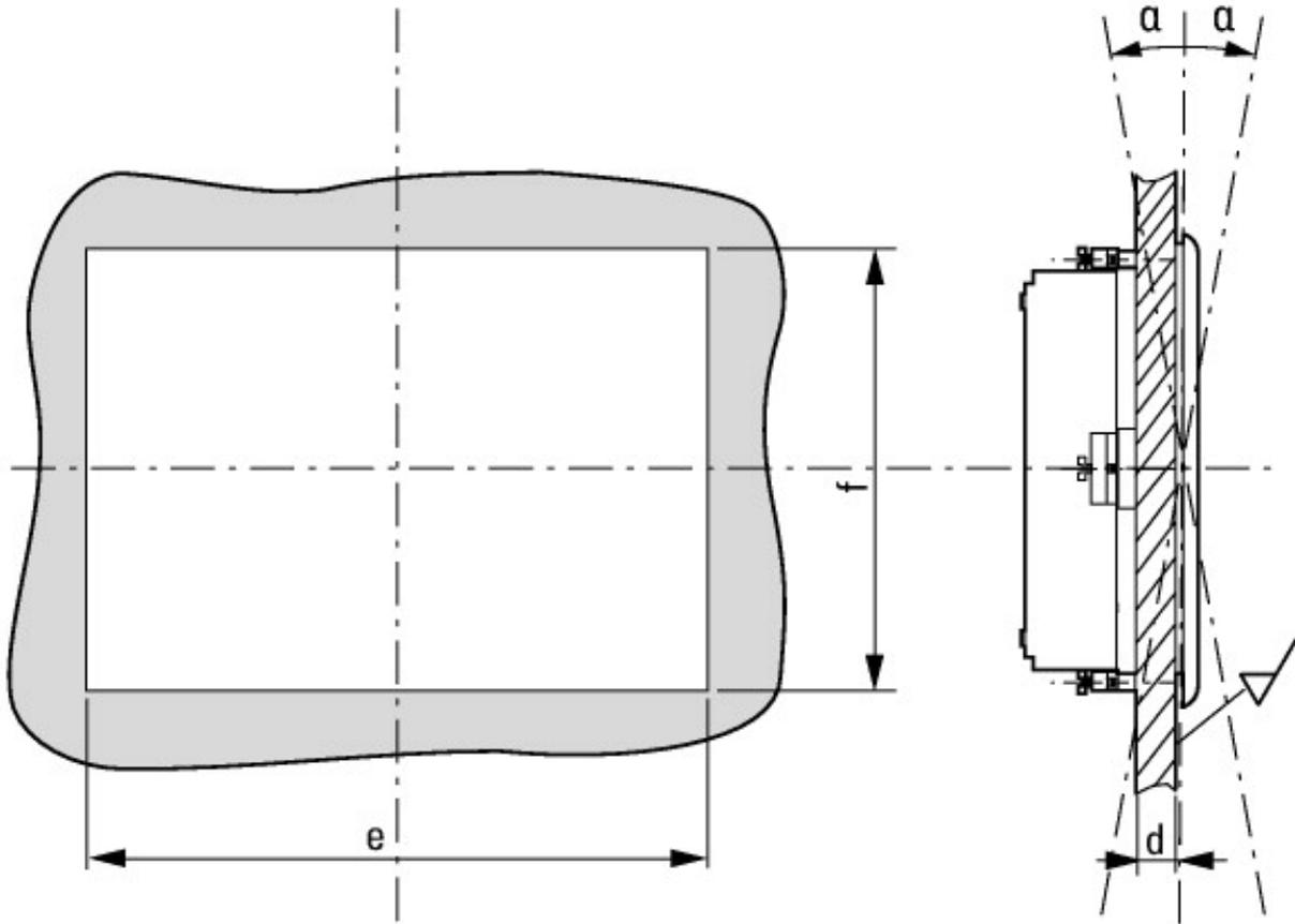
$1.5 \text{ mm} \leq d \leq 4 \text{ mm}, e = 388 \text{ mm}, f = 239 \text{ mm}, \# = 10^\circ$
