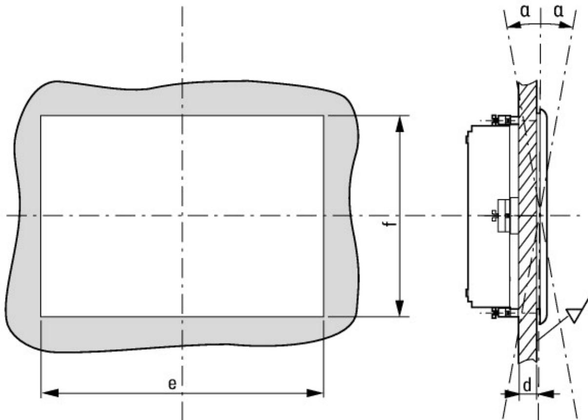
$2 \text{ mm} \leq d \leq 5 \text{ mm}, e = 183 \text{ mm}, f = 122 \text{ mm}, \# = 45^\circ$
