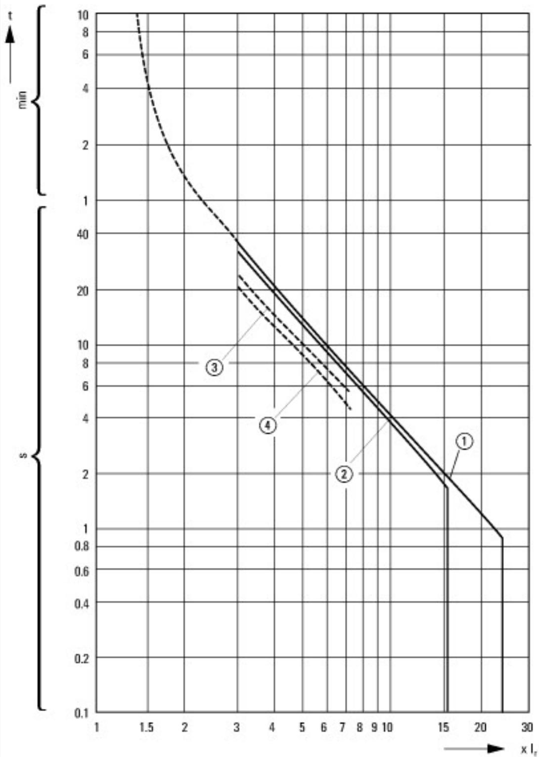
Tripping characteristics motor circuit breaker PKZM0-..., PKZM01
