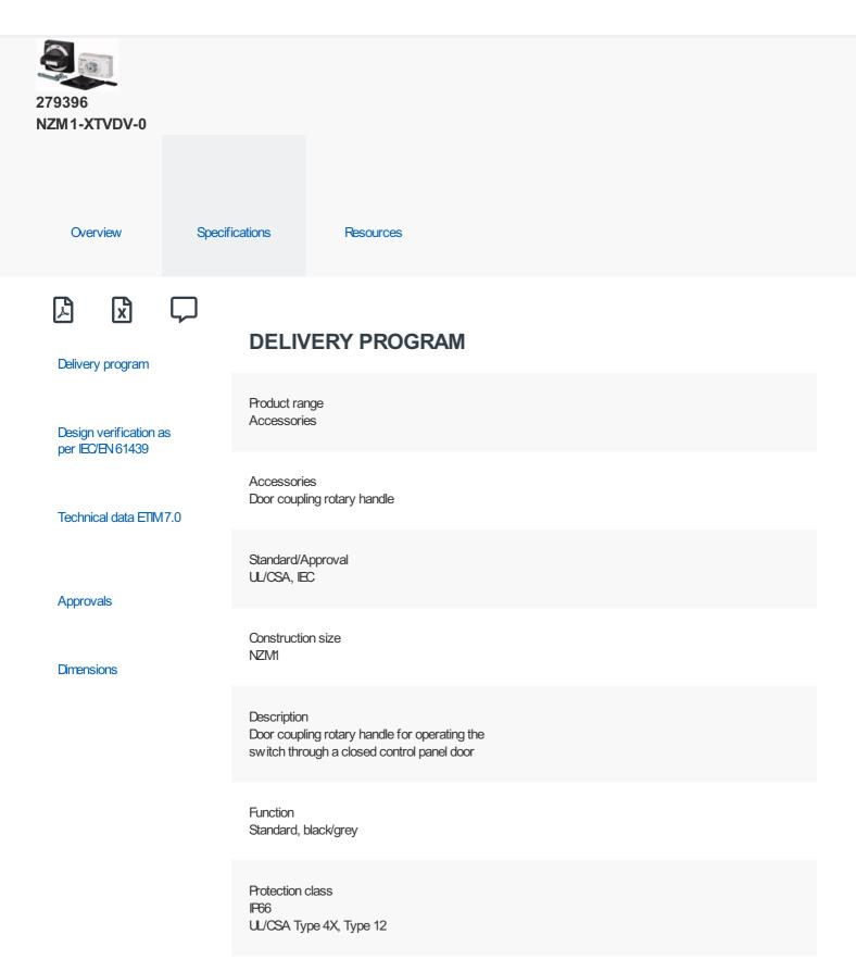
Locking facility lockable on the handle on the switch using up to 3 padlocks Modifiable on handle in I position as well With door interlock
