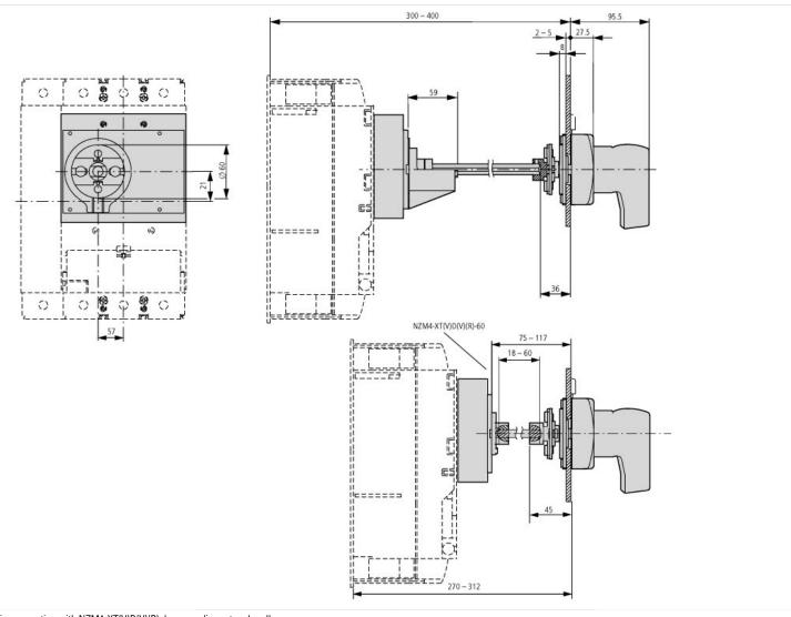
in connection with NZM4-XT(V)D(V)(R) door coupling rotary handle
