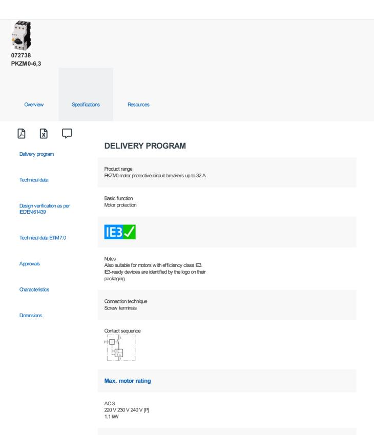
AC-3 380 V 400 V 415 V [P] 2.2 kW AC-3 440 V [P] 3 kW
