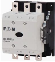
**Contactor, 380 V 400 V 90 kW, 2 N/O, 2 NC, RDC 24: 24 - 27 V DC, DC operation, Screw connection**
