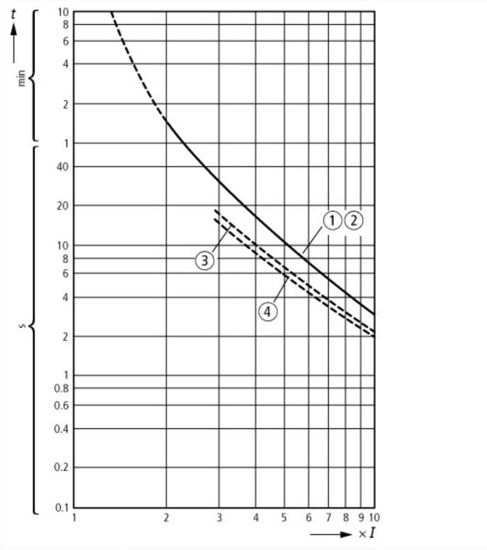
These tripping characteristics are mean values of the spread at 20 °C ambient temperature in a cold state. Tripping time depends on response current.
