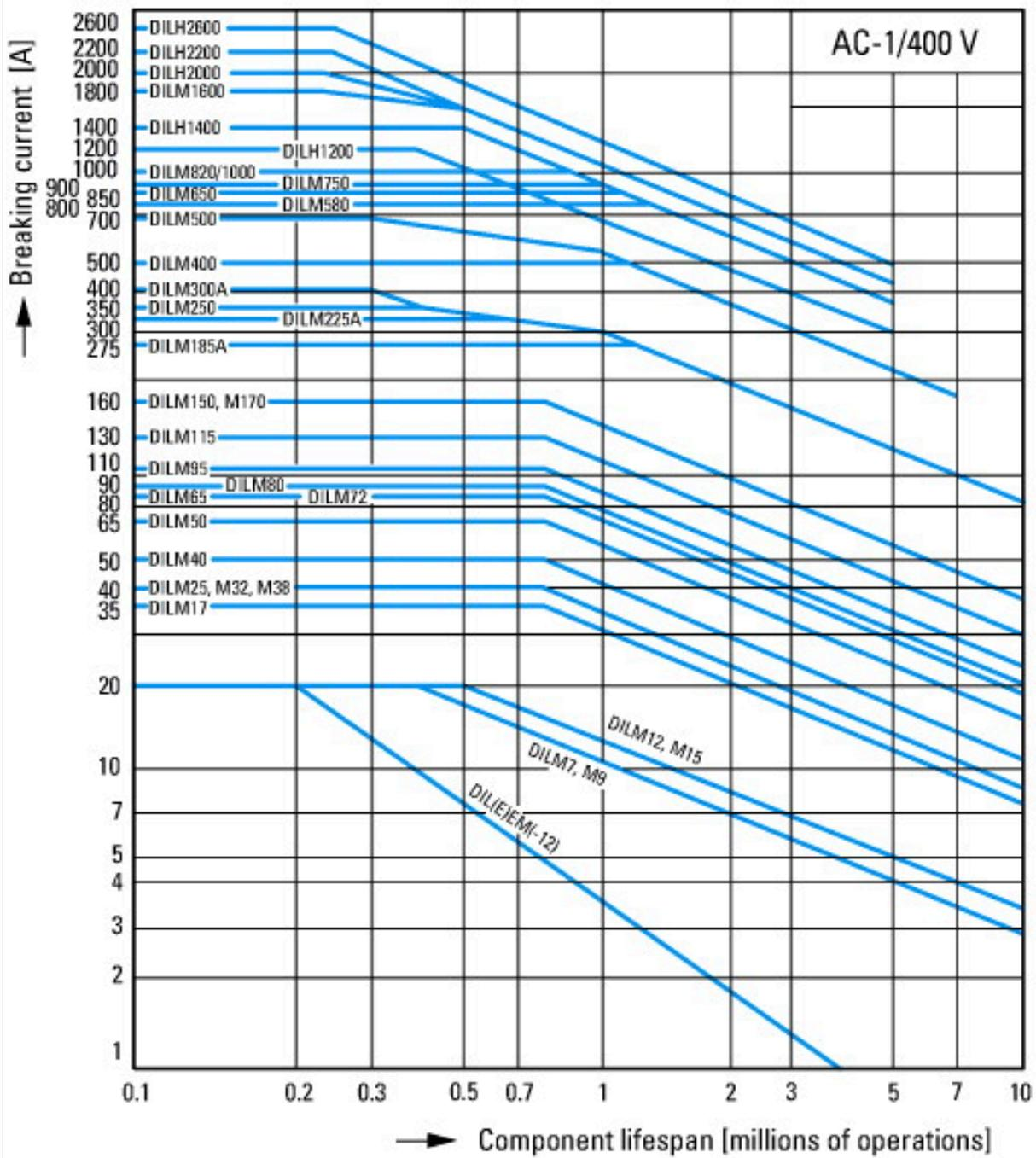
Switching conditions for 3 pole, non-motor loads
