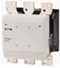
**Contactor, I<sub>th</sub> = I<sub>e</sub>: 1714 A, RAW 250: 230 - 250 V 50 - 60 Hz/230 - 350 V DC, AC and DC operation, Screw connection**
