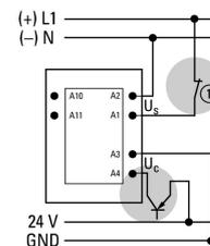
Low-power actuating devices such as PCB relays, actuating devices or position switches can be directly connected to A10/A11.
