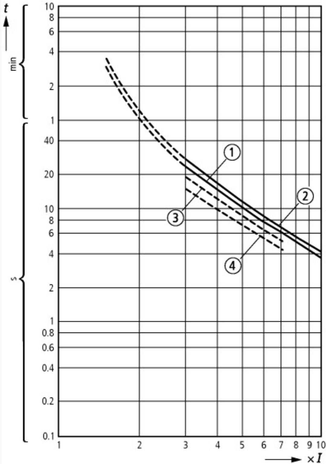
These tripping characteristics are mean values of the spreads at 20 °C ambient air temperature in a cold state.
