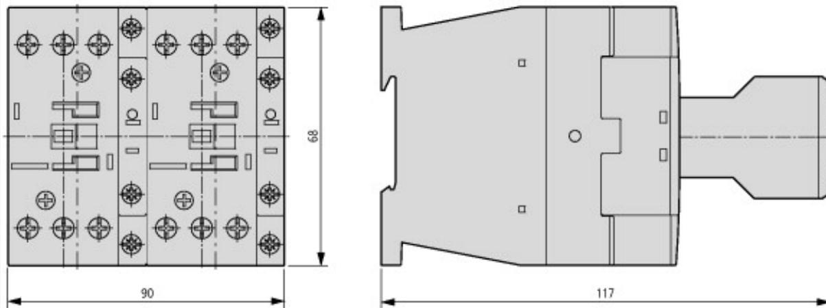
Basic unit with auxiliary contact module
