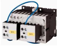
Reversing contactor combination, 380 V 400 V: 4 kW, 230 V 50 Hz, 240 V 60 Hz, AC operation
