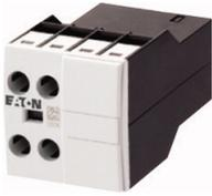
**Auxiliary contact module, Type: Front mounting auxiliary contact, 2 pole, I<sub>th</sub>= 16 A, 1 N/O, 1 NC, Front fixing, Screw terminals**
