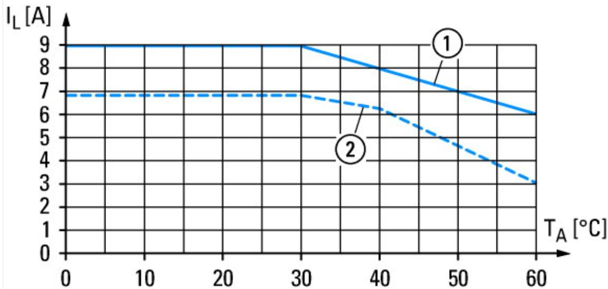
Electricity derating devices with  $I_o = 9$  A
