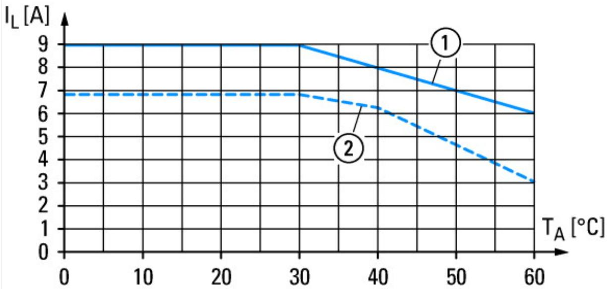
Electricity derating devices with  $I_e = 9$  A
