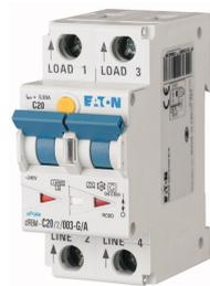
**Digital residual current circuit-breaker/miniature circuit-breaker, 20A, 30mA, miniature circuit-breaker trip curve: C, 2 p, residual current circuit-breaker trip characteristic: G/A**
