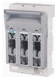
**NH fuse-switch 3p flange connection M10 max. 150 mm<sup>2</sup>; mounting plate; NH1**
