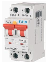
**Electronic RCD/MCB combination, 10 A, 100 mA, MCB trip characteristic: C, 2p, RCD trip characteristic: F**
