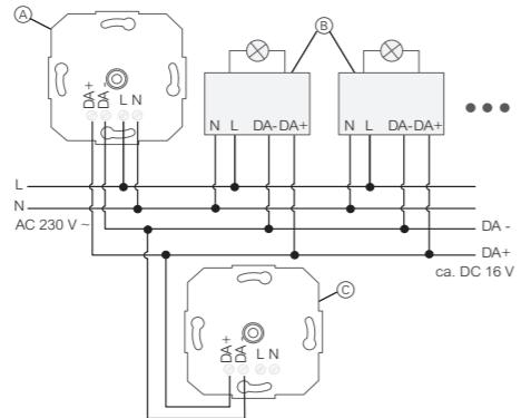
**(A)** DALI Rotary dimmer with connection to mains voltage: active operation
