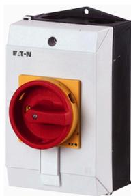
**Main switch, 3 pole + 1 N/O, 20 A, Emergency-Stop function, 90 °, Lockable in the 0 (Off) position, surface mounting**
