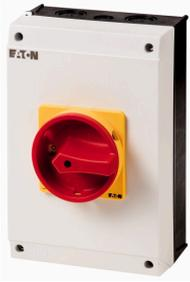
**Main switch, 6 pole + 1 N/O + 1 N/C, 63 A, Emergency-Stop function, 90 °, Lockable in the 0 (Off) position, surface mounting**
