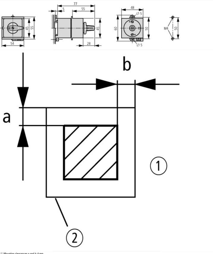
① Mounting clearances a and b: 4 mm ② exposed conductive part (metal)
