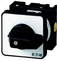
Reversing switches, Contacts: 5, 20 A, front plate: 1>0<2, 45 °, momentary, flush mounting
