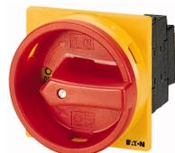
**Main switch, 3 pole, 32 A, Emergency-Stop function, Lockable in the 0 (Off) position, flush mounting**
