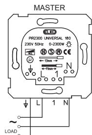
All → "arrow out" outputs of the slaves should be connected to the masters input 1
