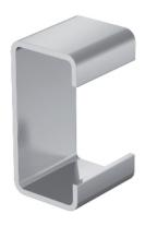
For static reasons, the spacer is always used to increase stability to prevent the support from deforming when the bracket is tightened with the hexagonal bolts. Spacer for use in U 5 support and in the head plate, type KU 7 VQP.
