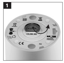
Open the battery compartment by using a coin to unscrew the cover counterclockwise to replace the rechargeable battery.
