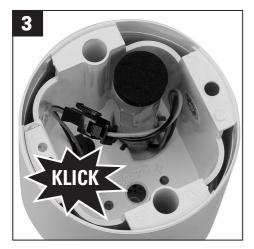
To do this, simply push the plug of the battery into the socket of the wireless doorbell until it audibly clicks into place. Please note the polarity (same colours to each other).
