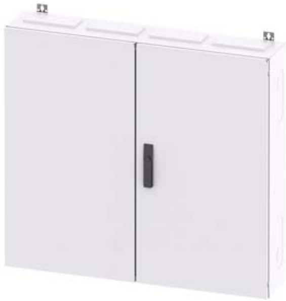
ALPHA 400 DIN, WALL-MOUNTING DISTRIBUTOR, AP-CUBICLE, RAL 9016, IP43, SK1, H=950 W=1050 D=210
