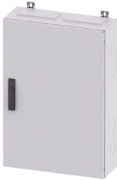
ALPHA 400 DIN, WALL-MOUNTING DISTRIBUTOR, DELIVERY FORM FLAT PACK, AP-CUBICLE, RAL 9016, IP43 SK2, H=800 W=550 D=210
