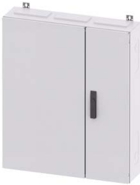
ALPHA 400 DIN, WALL-MOUNTING DISTRIBUTOR, DELIVERY FORM FLAT PACK, AP-CUBICLE, RAL 9016, IP43, SK1, H=950 W=800 D=210
