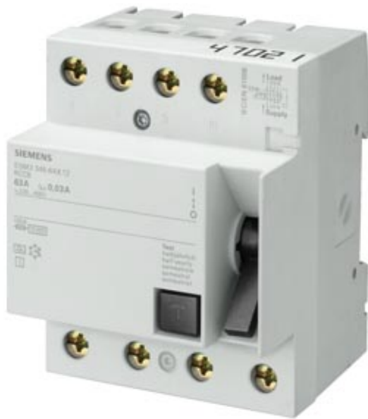
RES.CURRENT OP.CIRCUIT BREAKER TYPE A PSE/SSF 40A 3+N-POL IFN 30MA 400V 4MW 50-400HZ
