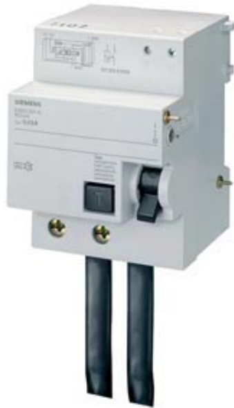
RC UNIT FOR MCB 5SX6+7 IMP WITHST STRGTH/SURGE STRGTH 80/100A 2POLE IFN 0.3A 230V FOR SELECTIVE SWITCH-OFF
