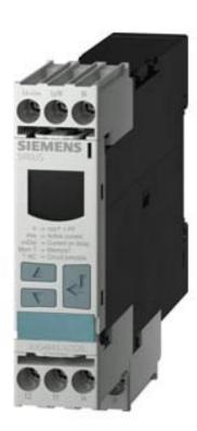
DIGITAL MONITORING RELAY COS-PHI A. CURRENT MONITORING FROM 90 TO 690V AC OVERSHOOT AND UNDERSHOOT INTERNAL POWER SUPPLY AC 50 TO 60 HZ SPIKE DELAY 0.1 TO 20S HYSTERESIS W. (I) 0.1 TO 2A 2 CHANGEOVER CONTACTS W. OR W/O ERROR LOG SCREW TERMINAL REPLACEMENT PRODUCT F. 3UG3014
