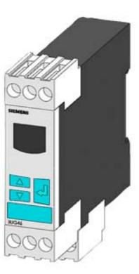
DIGITAL MONITORING RELAY VOLTAGE MONITORING, 22.5MM FROM 10 TO 600V AC/DC OVERSHOOT AND UNDERSHOOT SUPPLY VOLTAGE: AC/DC 24V DC AND AC 50 TO 60 HZ NO GALVANIC ISOLATION FROM MEASURING CIRCUIT INTERF. PEAK DELAY 0.1 TO 20S HYSTERESIS 0.01 TO 300V 1 CO CONTACT W. OR W/O ERROR LOG SCREW TERMINAL REPLACEMENT PRODUCT FOR 3UG3532-1AC..
