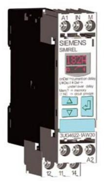
DIGITAL MONITORING RELAY CURRENT MONITORING, 22.5MM FROM 0.05 TO 10A AC/DC OVERSHOOT A. UNDERSHOOT AC/DC 24 TO 240V DC AND AC 50 TO 60 HZ ON AND SPIKE DELAY 0.1 TO 20S HYSTERESIS 0.01 TO 5A 1 CO CONTACT W. OR W/O ERROR MEMORY SCREW CONNECTION REPLACEMENT PRODUCT FOR 3UG3522-1AL20, 3UG3522-1AG20 AND 3UG3522-1AC48-0AA1
