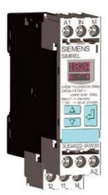
DIGITAL MONITORING RELAY CURRENT MONITORING, 22.5MM FROM 0.05 TO 10A AC/DC OVERSHOOT AND UNDERSHOOT SUPPLY VOLTAGE: AC/DC 24V DC AND AC 50 TO 60 HZ NO GALVANIC ISOLATION FROM MEASURING CIRCUIT STARTUP AND INTERF. PEAK DELAY 0.1 TO 20S HYSTERESIS 0.01 TO 5A 1 CO CONTACT W. OR W/O ERROR LOG SCREW TERMINAL REPLACEMENT PRODUCT FOR 3UG3522-1AC..
