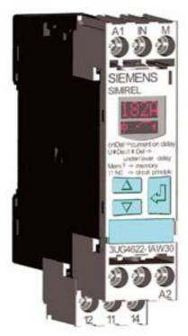
DIGITAL MONITORING RELAY CURRENT MONITORING, 22.5MM FROM 2 TO 500MA AC/DC OVERSHOOT A. UNDERSHOOT AC/DC 24 TO 240V DC AND AC 50 TO 60 HZ ON AND SPIKE DELAY 0.1 TO 20S HYSTERESIS 0.1 TO 250MA 1 CO CONTACT W. OR W/O ERROR MEMORY SCREW CONNECTION REPLACEMENT PRODUCT FOR 3UG3521-1AL20, 3UG3521-1AG20 AND 3UG3521-1AC48-0AA1
