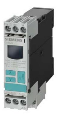
DIGITAL MONITORING RELAY CURRENT MONITORING, 22.5MM FROM 2 TO 500MA AC/DC OVERSHOOT AND UNDERSHOOT SUPPLY VOLTAGE: AC/DC 24V DC AND AC 50 TO 60 HZ NO GALVANIC ISOLATION FROM MEASURING CIRCUIT STARTUP AND INTERF. PEAK DELAY 0.1 TO 20S HYSTERESIS 0.1 TO 250MA 1 CO CONTACT W. OR W/O ERROR LOG SCREW TERMINAL REPLACEMENT PRODUCT FOR 3UG3521-1AC..
