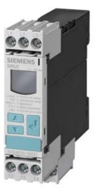
DIGITAL MONITORING RELAY UNBALANCE 0-20% REVERSIBLE PHASE SEQUENCE PHASE FAILURE 3X 160 TO 690V AC 50 TO 60 HZ UNDERVOLTAGE 160-690V HYSTERESIS 1-20V ON AND OFF DELAY 0-20S 2 CHANGEOVER CONTACTS SCREW TERMINAL REPLACEMENT PRODUCT FOR 3UG3012-1A...
