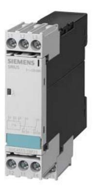
ANALOG MONITORING RELAY PHASE SEQUENCE MONITORING 3X 160 TO 260V AC 50 TO 60 HZ 2 CHANGEOVER CONTACTS SCREW TERMINAL REPLACEMENT PRODUCT FOR 3UG3511-1BQ50
