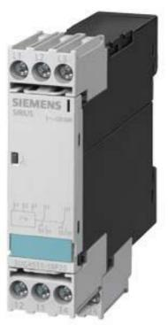
ANALOG MONITORING RELAY PHASE SEQUENCE MONITORING 3X 160 TO 260V AC 50 TO 60 HZ 1 CHANGEOVER CONTACT SCREW TERMINAL REPLACEMENT PRODUCT FOR 3UG3511-1AQ50 OR 3UG3511-1AV50
