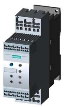
SIRIUS SOFT STARTER, S0, 38A, 18.5KW/400V, 40 DEGR., AC 200-480V, AC/DC 24V, SPRING-LOADED TERMINALS
