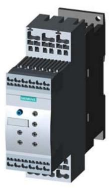
SIRIUS SOFT STARTER, S0, 12.5A, 5.5KW/400V, 40 DEGR., AC 200-480V, AC/DC 24V, SPRING-LOADED TERMINALS
