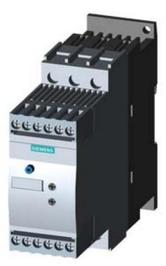
SIRIUS SOFT STARTER, SIZE S0, 38A, 18.5KW/400V, 40 DEGREES, 200-480V AC, 24V AC/DC, SCREW TERMINALS
