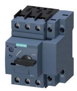
CIRCUIT-BREAKER SZ S0, FOR MOTOR PROTECTION, CLASS 10, W. OVERLOAD RELAY FUNCTION A-RELEASE16...22A, N-RELEASE 286 A, SCREW CONNECTION, STANDARD SW. CAPACITY
