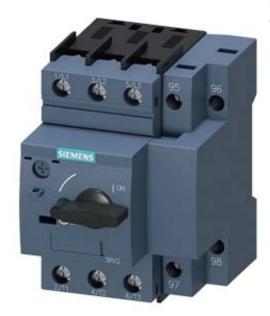
CIRCUIT-BREAKER SZ S0, FOR MOTOR PROTECTION, CLASS 10, W. OVERLOAD RELAY FUNCTION A-RELEASE 10...16A, N-RELEASE208A, SCREW CONNECTION, STANDARD SW. CAPACITY
