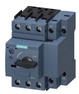
CIRCUIT-BREAKER SZ S00, FOR MOTOR PROTECTION, CLASS 10, W. OVERLOAD RELAY FUNCTION A-RELEASE 2.8A...4A, N-RELEASE 52A, SCREW CONNECTION, STANDARD SW. CAPACITY
