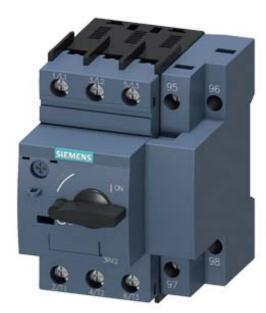
CIRCUIT-BREAKER SZ S00, FOR MOTOR PROTECTION, CLASS 10, W. OVERLOAD RELAY FUNCTION A-RELEASE 0.45...0.63A, N-RELEASE8.2A SCREW CONNECTION, STANDARD SW. CAPACITY
