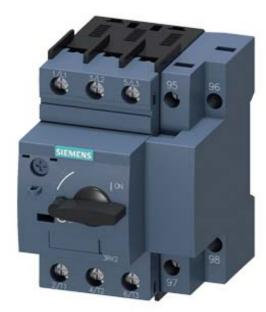
CIRCUIT-BREAKER SZ S00, FOR MOTOR PROTECTION, CLASS 10, W. OVERLOAD RELAY FUNCTION A-RELEASE 0.28...0.4A,N-RELEASE 5.2A SCREW CONNECTION, STANDARD SW. CAPACITY
