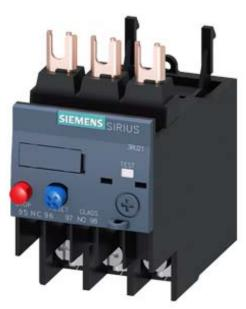
OVERLOAD RELAY 3.5...5.0 A FOR MOTOR PROTECTION SZ S0, CLASS 10, F. MOUNTING ONTO CONTACTOR MAIN CIRCUIT: RING CABLE LUG AUX. CIRCUIT: RING CABLE LUG MANUAL-AUTOMATIC-RESET
