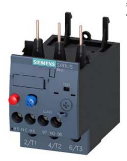
OVERLOAD RELAY 3.5...5.0 A FOR MOTOR PROTECTION SZ S0, CLASS 10, F. MOUNTING ONTO CONTACTOR MAIN CIRCUIT: SCREW TERMINAL AUX. CIRCUIT: SCREW TERMINAL MANUAL-AUTOMATIC-RESET
